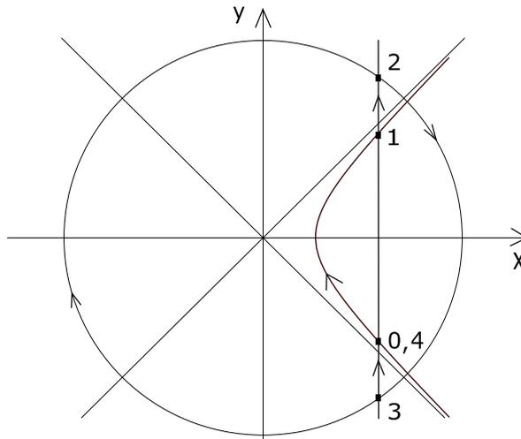
Figure 3.3: Trajectories corresponding to a  $T$ -periodic solution.
