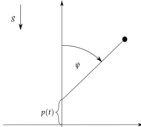
Figure 2.1: Vertically excited inverted pendulum.
