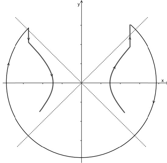
Figure 2.3: The phase space of the inverted pendulum, if  $\omega_h > \omega_e$ .
