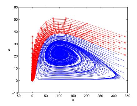
Figure 3.5: Phase portrait of system (3.6) with different initial position when n = 25. The dotted red line show the manifold go to (0,0) at last and the blue show the manifold go to limit cycle of system (3.6) around the equilibrium  $P^*$ . The parameter values a = 5, b = 1, k = 0.01, e = 0.2, d = 1,  $\lambda = 0.1$ .
