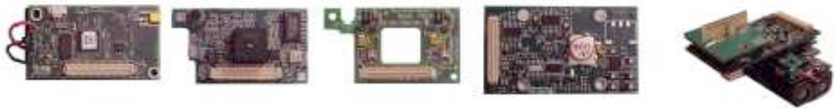
Fig. 6. Sensor hardware from left to right: (a) Mica2 network node, (b) Mica Sensor Board, (c) Mica Power Board, (d) TWR-ISM-002 Radar Board, and (e) All of the boards attached together.
